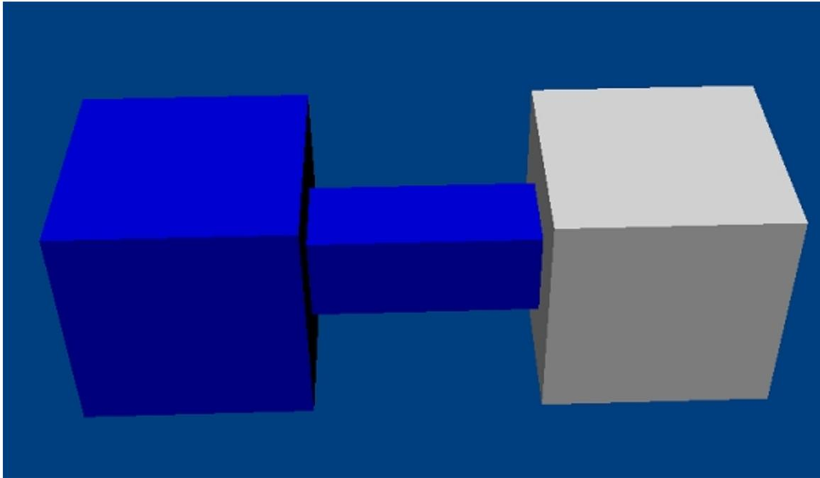
The fixed joint effectively glues two bodies together with no remaining degrees of freedom for relative motion. It is useful to set it to be breakable (see [Breakable Joint](#)) to simulate simple fracture effects.
