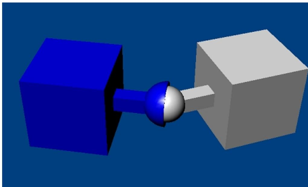
A spherical joint is the simplest kind of joint. It constrains two points on two different bodies from coinciding. This point, located in world space, is the only parameter that has to be specified (the other parameters are optional). Specifying the anchor point (point that is forced to coincide) in world space guarantees that the point in the local space of each body will coincide when the point is transformed back from local into world space.
