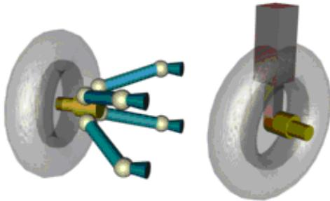
The figure shows a real mechanical component (single wheel suspension of a car) made up of a large number of joints, and an alternative simpler scheme with about the same degrees of freedom.
