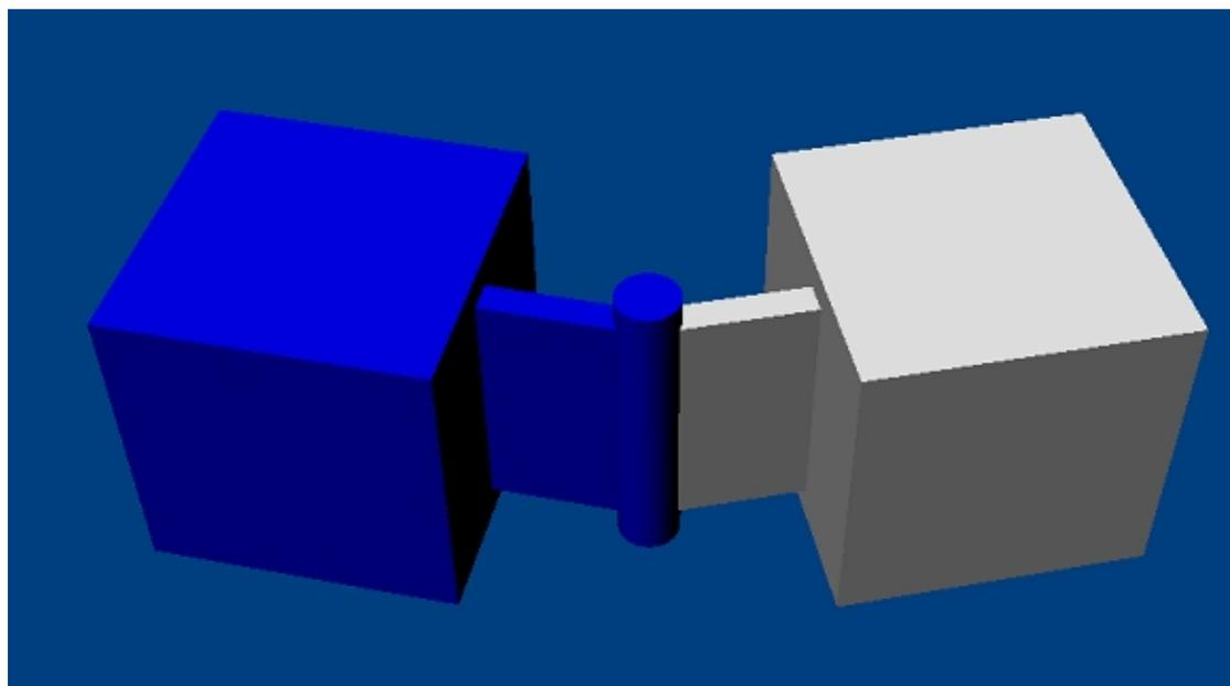
A revolute joint removes all but a single rotational degree of freedom from two objects. The axis along which the two bodies may rotate is specified with a point and a direction vector. In theory, the point along the direction vector does not matter, but in practice, it should be near the area where the bodies are closest to improve simulation stability.
