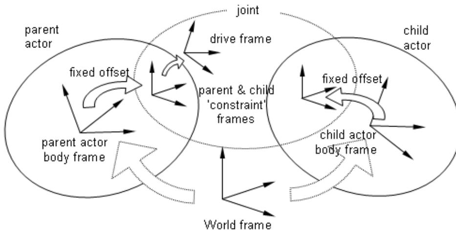
The joint frames are sketched separate from each other for clarity, but the joint constraints will act to bring the two constraint frames together and drive constraints will act to bring the drive frame and the child frame together.
