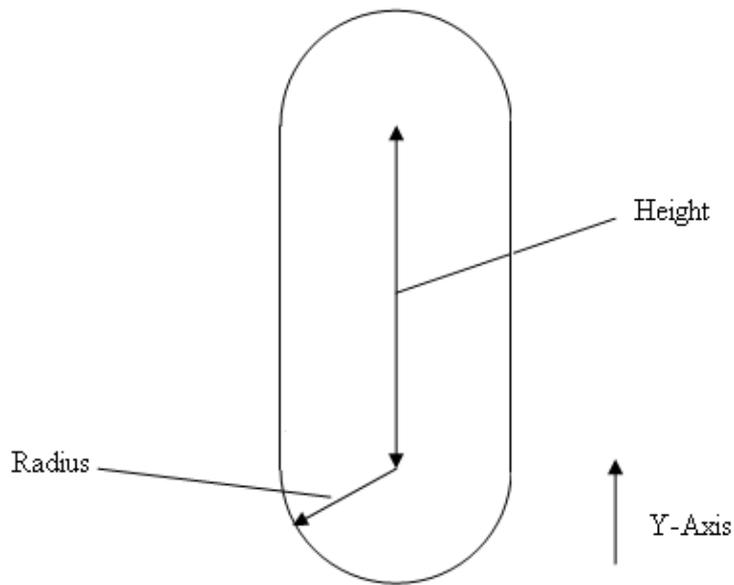
Capsules (class `NxCapsuleShape`), also called line swept spheres, are like cylinders that have rounded ends. Capsules are great to approximate round shapes like body parts because their collision detection is very fast and robust, even more so than boxes. The image below shows a character whose bounding boxes are made using capsules.
