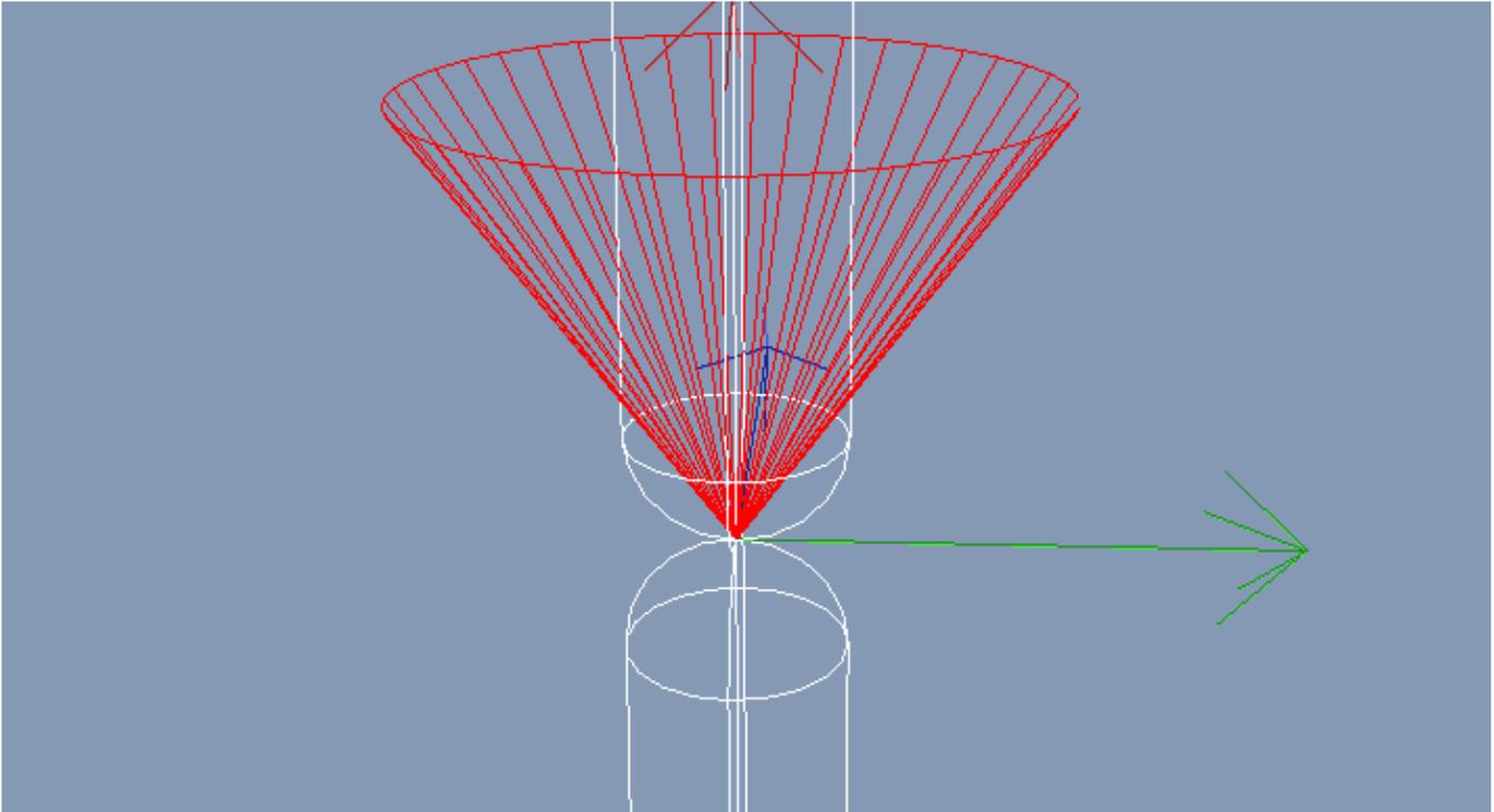
In the above screen shot, the cone is represented in red. The principal child axis (x-axis) is a red arrow near the center of the cone; it is constrained to lie within the cone.
