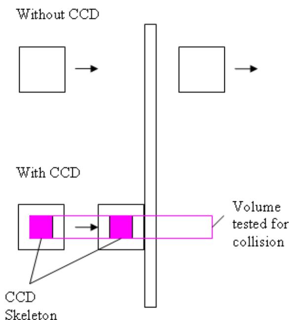
In the current version of the SDK, CCD is supported for dynamic vs. dynamic objects and dynamic vs. static objects.
