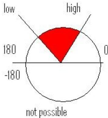
To achieve this configuration, it is necessary to rotate the joint counter-clockwise so that low is below the 180 degree line.
