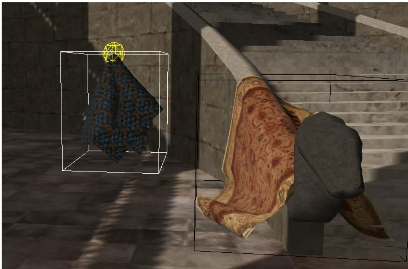
In a similar way to rigid bodies (see [rigid body sleeping](#)), cloths can go to sleep after a period of inactivity. The objective of sleeping is to improve performance by not simulating cloths which are not moving.
