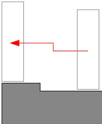
However, if the obstacle is too big (i.e., its height is greater than the *stepOffset* parameter), the controller can't climb automatically over, thus the character gets stuck (correctly this time):
