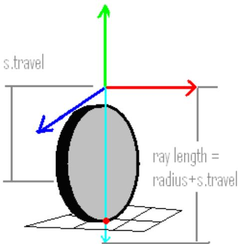
The meaning of the suspension `NxSpringDesc::targetValue` has also changed. It is now decoupled from the suspension travel, and is a value between 0 and 1 that determines at what % of whole travel the rest length of the spring should be, 0 mapping to the default of full extension along the suspension travel.
