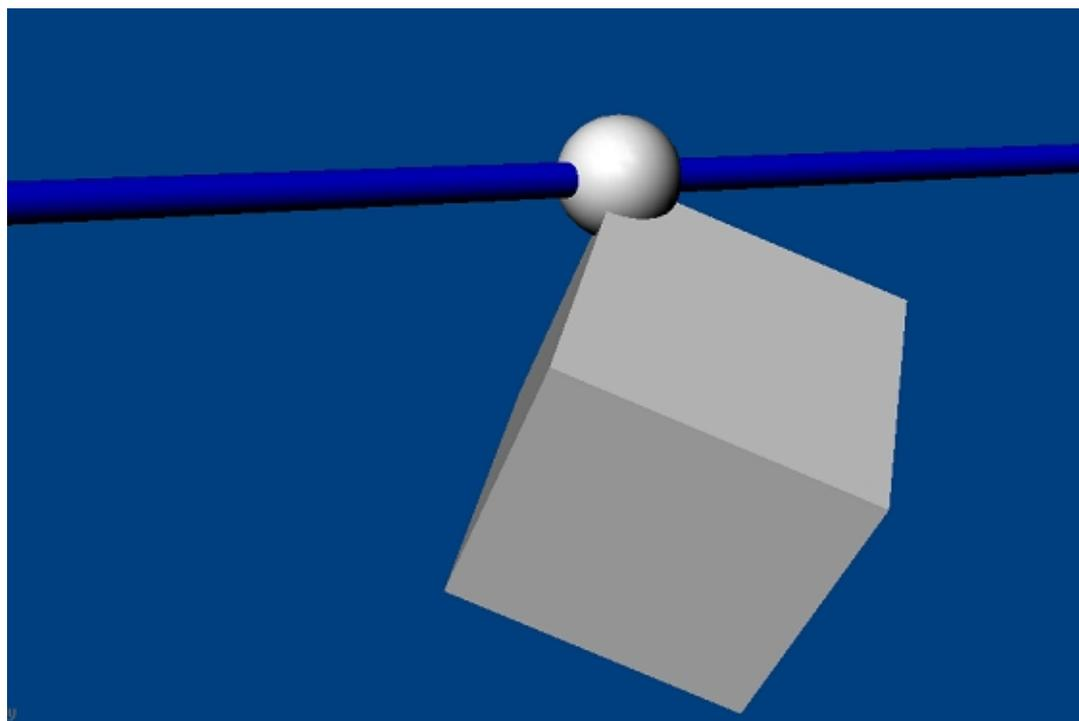
A point on line joint constrains a point on one actor to only move along a line attached to another actor. The point attached to the line is the anchor point for the joint. The line through this point is specified by its direction (axis) vector.
