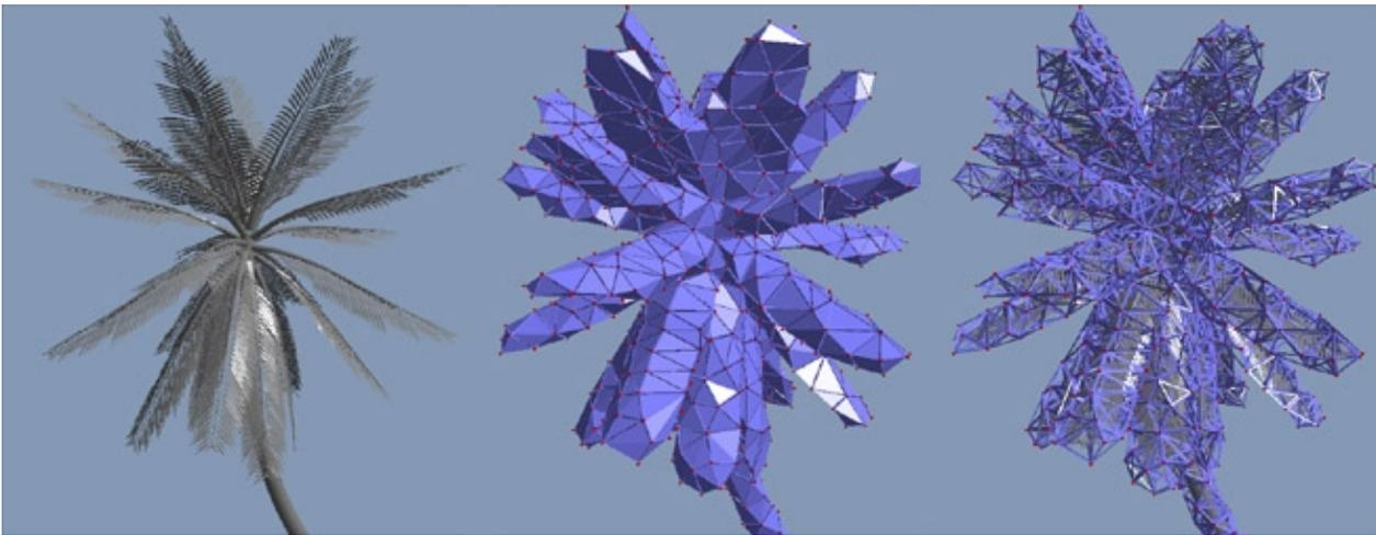
The resolution of the tetrahedral mesh can be chosen independently of the resolution of the triangle mesh. This allows for choosing a level of detail for the simulation without losing visual resolution. The following images show different resolutions of a palm tree mesh. With the coarser meshes, independent movement of individual leaves is not possible. To get this dynamic feature, more tetrahedra are needed as shown on the right:
