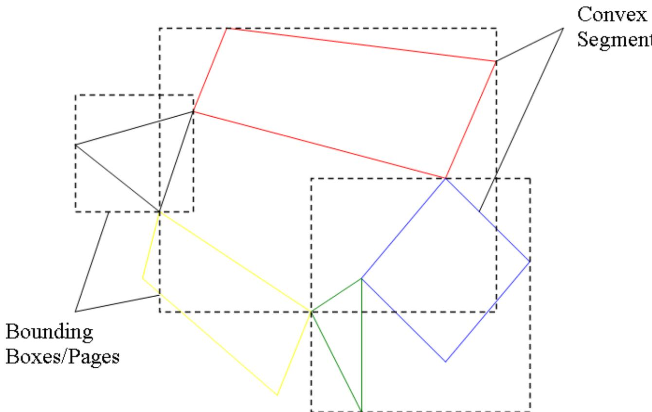
When the mesh is loaded into a hardware scene, the user can retrieve a bounding box for each mesh page, and use this information to upload appropriate pages to the card to support their simulation.
