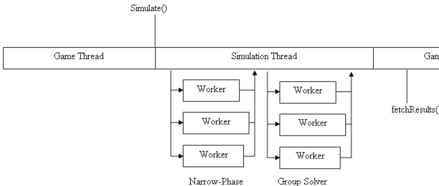
The SDK provides the following two distinct ways to control how work is scheduled between worker threads:
