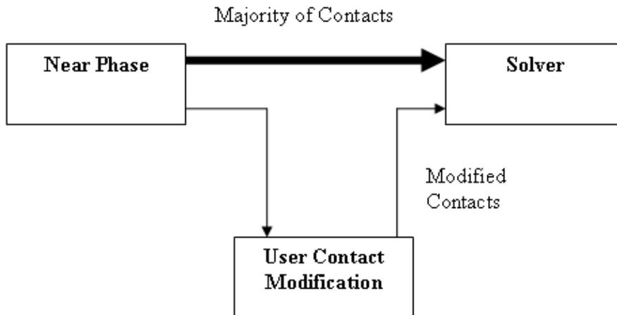
For example, it might be necessary to modify contacts when a car crosses a seam between two mesh objects. At this point, with default contact generation, incorrect contact constraints can be generated due to collision not being performed across both objects at once.
