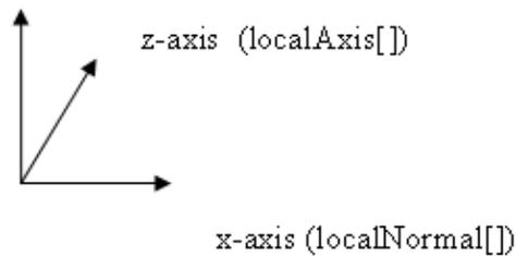
The first (X) basis vector of joint space is called the 'normal', the second (Z) is called the 'axis', and the third (Y) is called the 'binormal', computed as a cross product of the first two. The 'anchor' is the point where the frame is located. The word 'local' denotes that the frames are not in the world but rather in the actor space.
