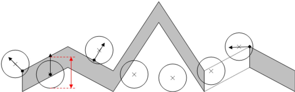
NOTE: An optimization in the sphere and capsule contact generation causes the heightfield not to generate contacts until the center of the sphere/capsule is in contact with the vertical extent of the heightfield. The same optimization also leads to spheres and capsules only generating contact points against edges if their centers are above the heightfield surface (see the examples above).
