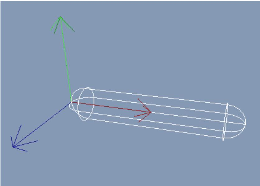
The red axis in the above screen shot is the twist axis, and the bone is represented as a capsule. The green and blue axes are the swing axes.
