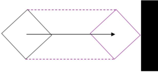
You can perform a sweep with a box shape by using the `NxScene::linearOBBSweep()` method. The results are returned via an `NxSweepQueryHit` structure.
