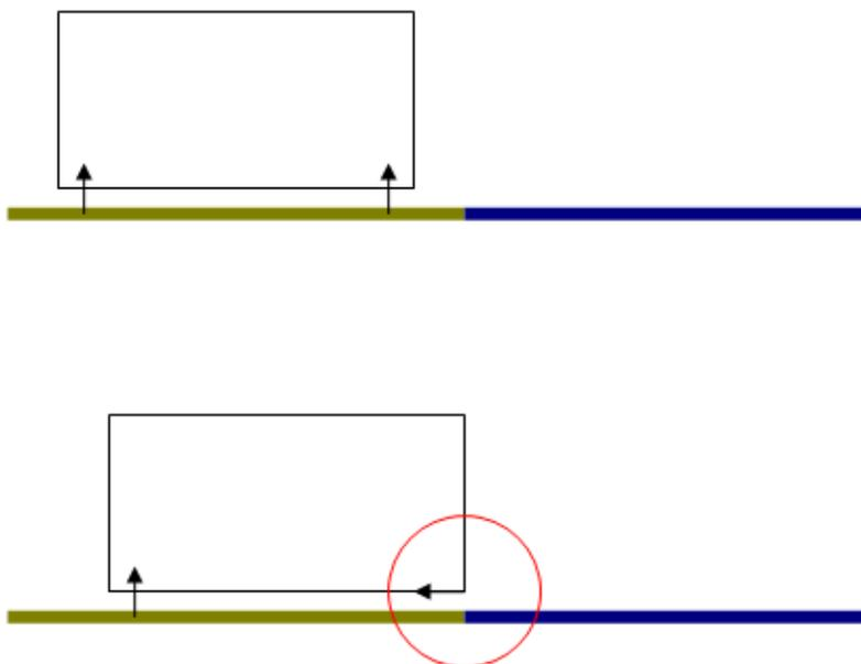
Contact modification is accomplished by providing a callback class which receives notifications when contacts are available to be modified.
