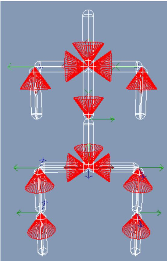
As soon as the key framed animation is turned off, notice that the skeleton folds up in an unrealistic manner. A real skeletal joint has anatomically imposed limits on its motion. To make the rag doll behave in a more realistic manner, it is necessary to approximate these limits.
