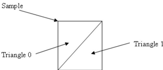
In addition to specifying the tessellation flag, the sample also defines the materials for each triangle in the quad. The triangles in the quad are numbered so that triangle 0 is always the triangle which shares an edge with the triangle to the right of the quad (see the diagram above). In this way, triangle numbering is independent of the tessellation flag.
