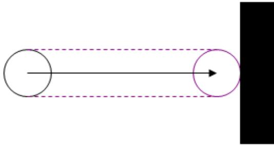
You can perform a sweep with a capsule shape by using the `NxScene::linearCapsuleSweep()` method. The results are returned via an `NxSweepQueryHit` structure.
