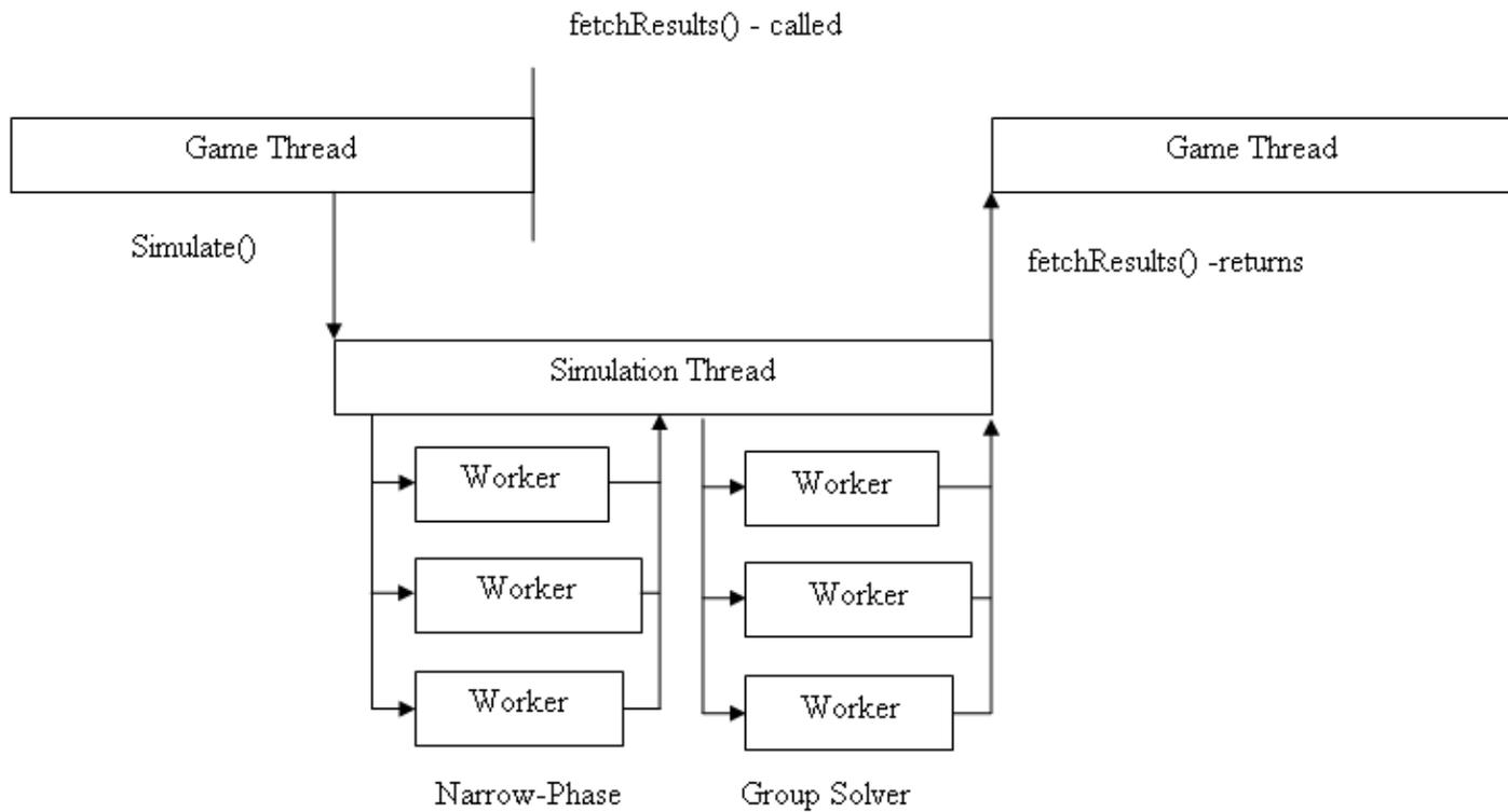
When NX\_SF\_SIMULATE\_SEPARATE\_THREAD is not specified, it is displayed as follows:
