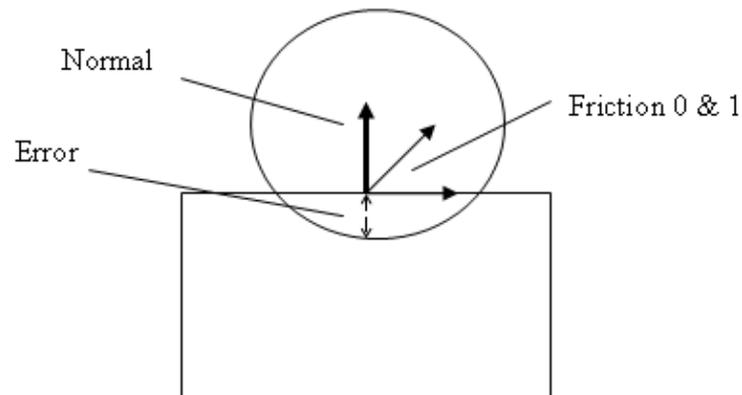
Contact modification can be enabled on a per actor basis using the `NX_AF_CONTACT_MODIFICATION` actor flag. This tells the SDK to call the contact modification callback for each contact between the actor and any other actor.
