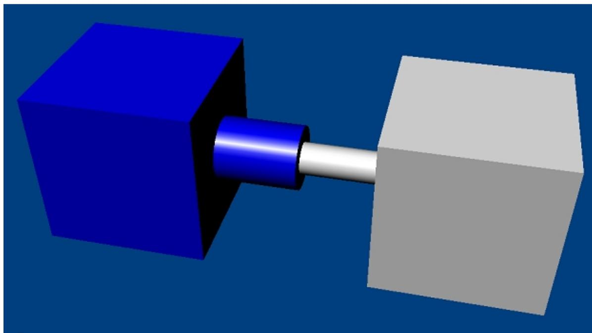
A cylindrical joint permits both relative translational and rotational movement between two bodies along a single axis (i.e., the bodies are allowed to both slide and twist along the axis of the joint). It is usually necessary to add joint limits to prevent the bodies from getting too far from each other along the joint axis. If the distance becomes too great, then the SDK can have difficulty maintaining the joint constraints (see [Joint Limits](#)).
