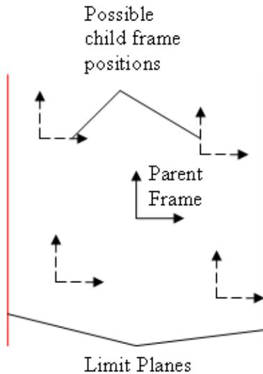
If one of the free DOFs is locked then the joint collapses to a planar joint and the origin of the child frame is constrained to lie between a pair of parallel lines centered in the selected plane of the parent frame.
