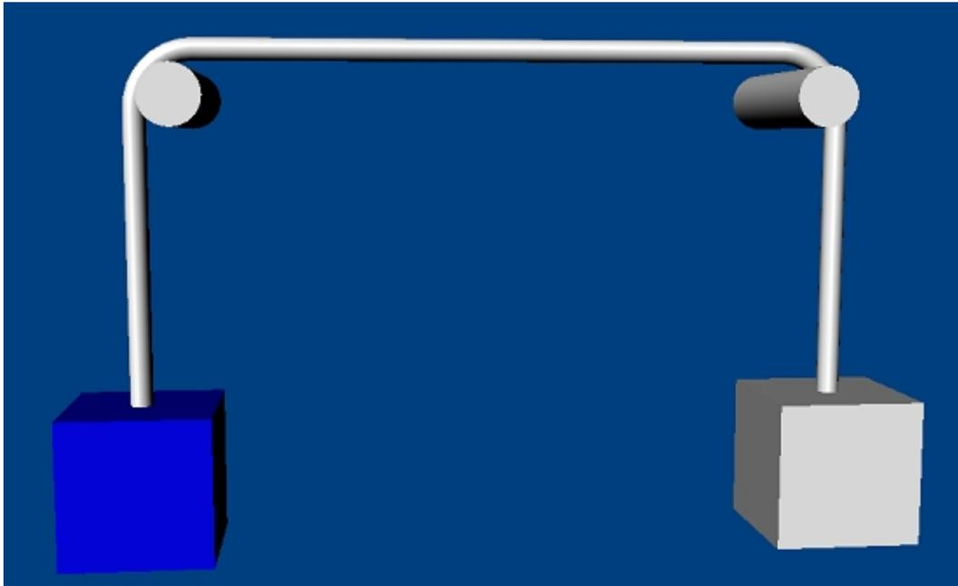
The pulley joint simulates a rope that can be thrown across a pair of pulleys. In this way, it is similar to the distance joint (the length of the rope is the distance) but the rope doesn't connect the two bodies along the shortest path, rather it leads from the connection point on one actor to the pulley point (fixed in world space), then to the second pulley point, and finally to the other actor.
