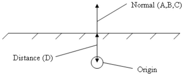
Planes (class `NxPlaneShape`) are useful for simple demos in which a ground plane is needed but little else. A plane is characterized in the world space plane equation with the following:
