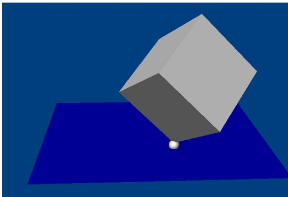
A point in plane joint constrains a point on one actor to only move inside a plane attached to another actor. The point attached to the plane is defined by the anchor point. The joint's axis specifies the plane normal.
