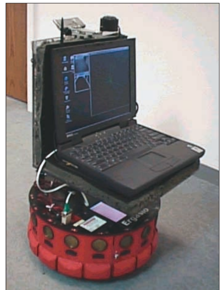
Figure 6. The hardware used by Cerebus. A commodity laptop with a USB frame grabber and an NTSC board camera mounted on a Real world Interface Magellan robot base.
