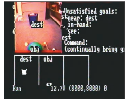
Figure 5. Kluge follows the command "continually bring green to blue." The parser binds the object role to the color green and the destination role to blue, then asserts the goals in-hand(object) and near(destination) . The robot grasps the green ball then drives toward the blue trash can.
